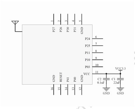
Note: There should be no circuitry directly above or below the module antenna.
