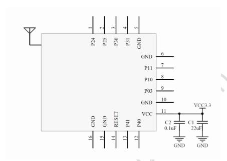
Note: There should be no circuitry directly above or below the module antenna.
