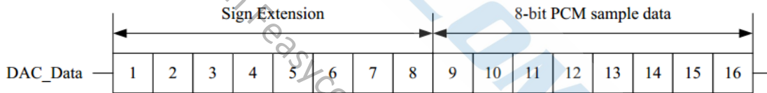
Figure 6: 16-Bit Output Data with 8-Bit PCM Sample Data and Sign Extension
